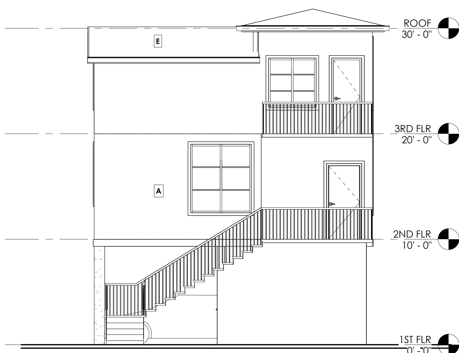
2 2 BED - TYPE C - EAST ELEVATION 3/16" = 1'-0"
