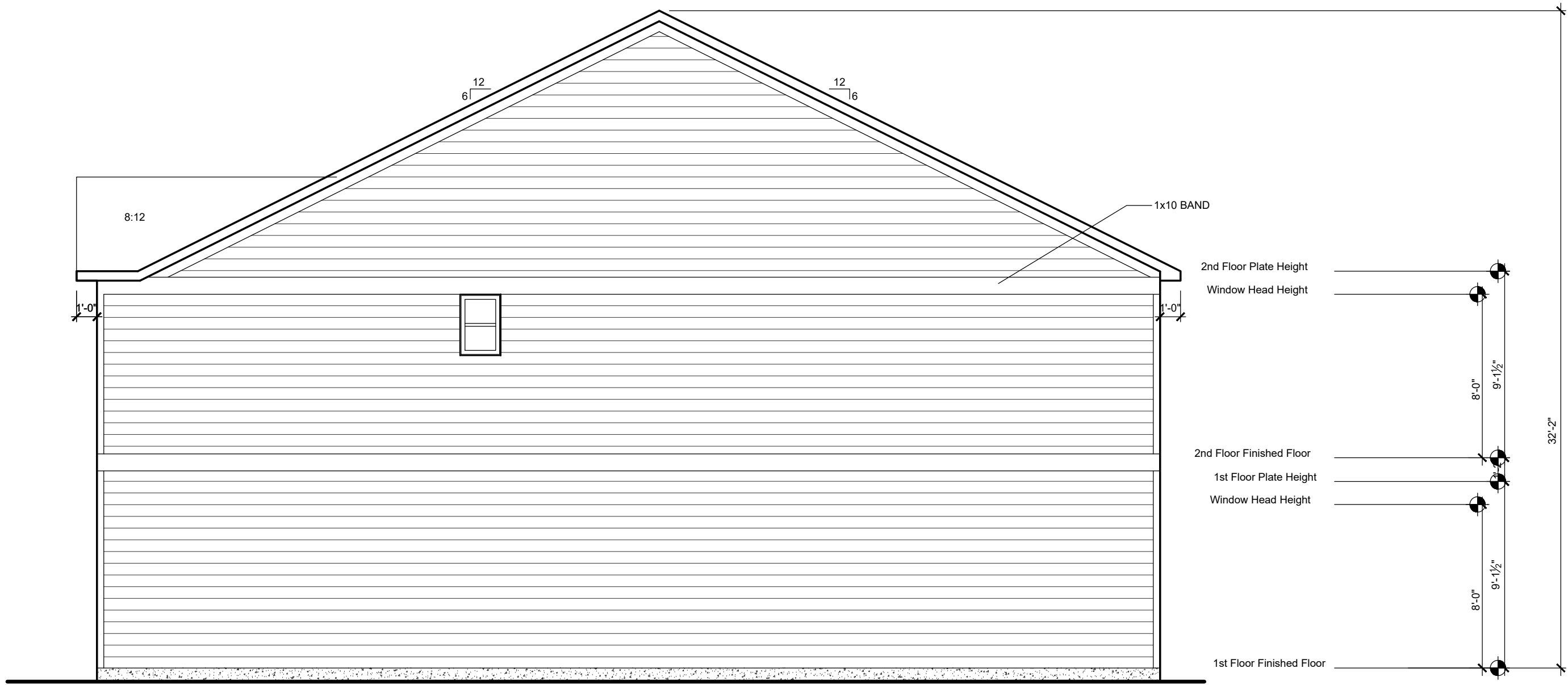
RIGHT SIDE ELEVATION SCALE: 3/32"=1'-0" (11x17" SHEET SIZE) SCALE: 3/16"=1'-0" (24x36" SHEET SIZE)
